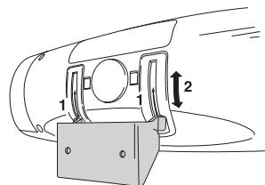
You can swivel the control unit on the wall bracket to adjust the angle. Locking the control unit ensures that it cannot be removed from the wall bracket when swivelled.
