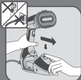
**EN** Unlock and remove the water tank.
