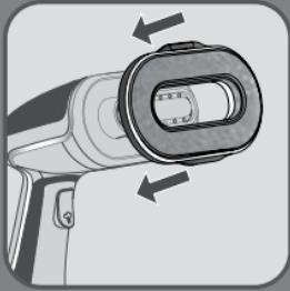
The CLEAN PAD\* is composed of one side with micro-fiber and the other side with lint & hair remover.
