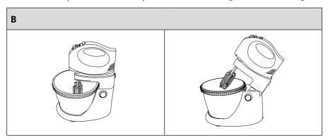
Press button (a) to release the lock of the motor unit (b) and with the other hand remove the motor unit (b). To release the attachments press button (a) and remove the attachments.
