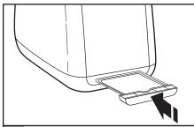
Return crumb tray to Toaster. Press it in firmly until it clicks into position. Do not use the Toaster without the crumb tray in proper position.
