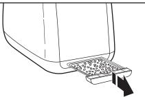
Press and release the center of the crumb tray then slide it out. Shake the crumbs into a waste container. It is recommended that the crumb tray be emptied after each use. The crumb tray can be washed in the top rack of a dishwasher.
