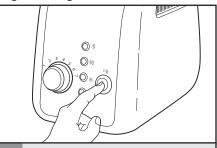
Press the TOAST/CANCEL (□♠) button to begin toasting. The centering racks will adjust automatically to hold food upright. When toasting is complete, the End-of-Cycle signal will beep, the Toaster will shut off and raise the toast.
