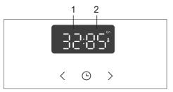
Turn the COOKING SYSTEM SELECTOR KNOB (hot air and lower heater). Symbol, preset temperature, current temperature, and set temperature will appear on the display. If the probe temperature is below 30 °C, the display will read "--: 80".
