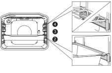
With telescopic extendible guides, first pull out the guides of one level and place the grid or the baking tray onto them. Then, push them in with your hand as far as they will go.
