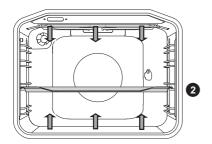
The heaters in the bottom and in the ceiling of the oven cavity will radiate heat evenly into the oven interior.
