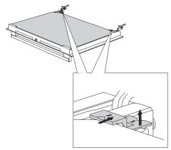
1 Slightly lift the supports on the left and right side of the door (marking 1 on the support) and pull them away from the glass pane (marking 2 on the support).
