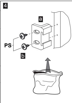
**Note:** Installation step for 2, screws for connecting top plastic part should not be screwed very hard, because of moving the plastic part easily left or right side.
